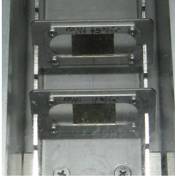
Figure 4.4: The ^{150}\text{Nd} targets used in the experiment, 1 \text{ mg/cm}^2 and 2 \text{ mg/cm}^2 .
